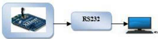
Fig 6. Receiver section (RTO)
